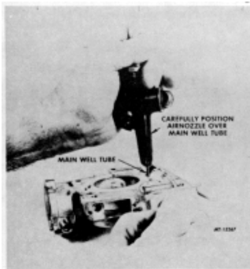
FIG. 20. Blowing Out Main Well Tube
