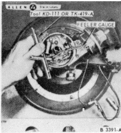
FIG. 10. Adjusting New Breaker Point Gap
